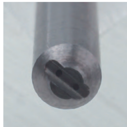
Shank end suitable for minimal quantity lubrication without build-up or dead pockets of coolant.
