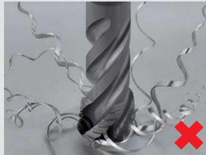
Thread chips can cause tool breakage
